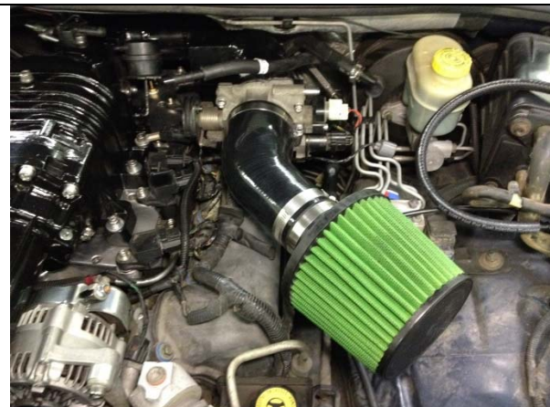
Figure 42: Air filter assembly attached to throttle body in correct orientation.
