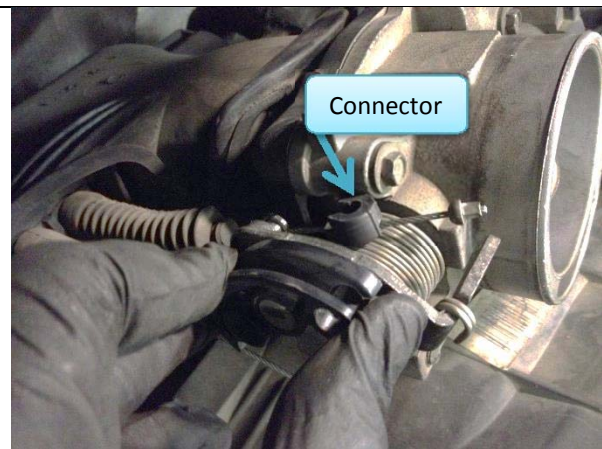
Figure 10: Cruise control connector after disconnecting.
