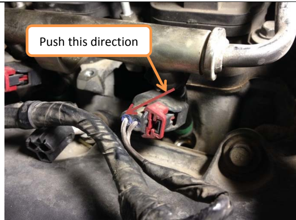
Figure 16: Fuel injector wire connectors.
