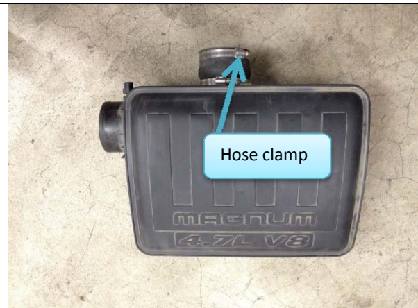
Figure 5: Upper intake after removal.
