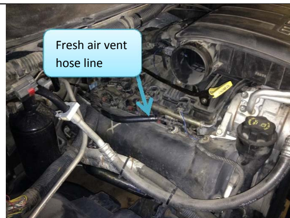
Figure 2: Filter housing and intake tube removed.
