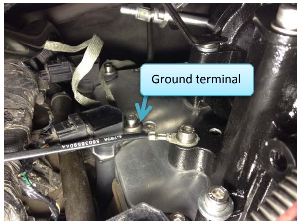
Figure 30: Ground wire terminal secured to coil pack.
