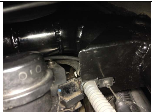
Figure 39: Throttle cables attached to bracket on intake tube.
