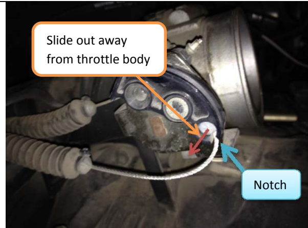
Figure 9: Throttle cable out of channel.
