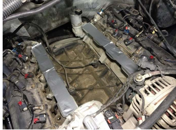
Figure 22: Intake ports covered.
