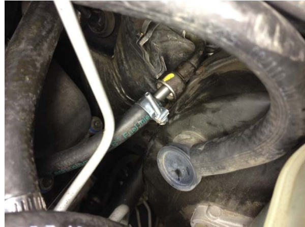
Figure 36: Fuel line extension attached to existing fuel line connection.
