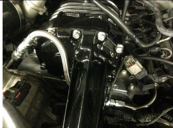
Figure 28: New fuel crossover hose in an "S" bend under supercharger nose.
