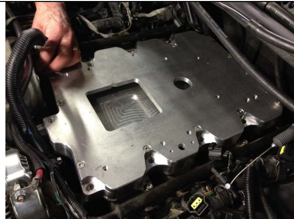
Figure 27: Intake tub assembly installed.
