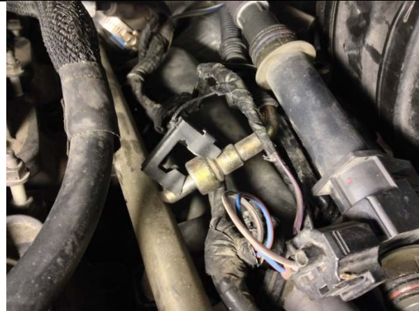
Figure 15: Fuel line safety clip after removal.
