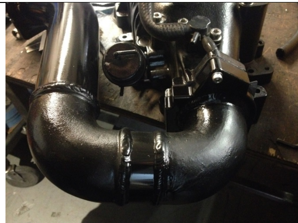
Figure 36: Non-EGR intake hose, sits on driver side.
