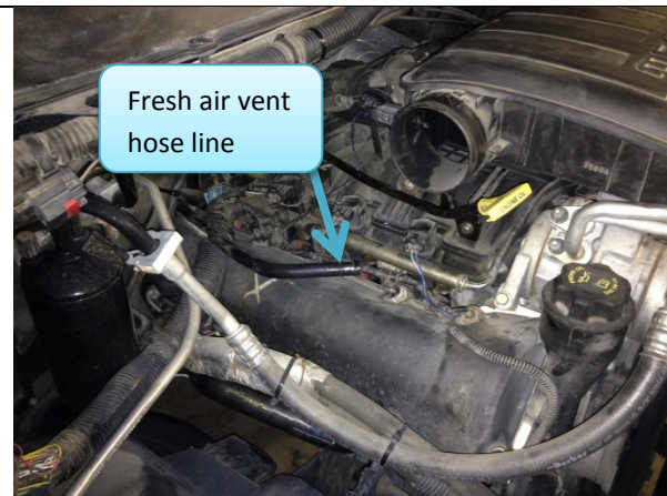
Figure 2: Filter housing and intake tube removed.
