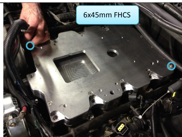
Figure 30: Intake tub assembly installed.
