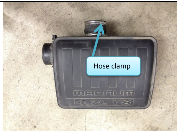
Figure 5: Upper intake after removal.
