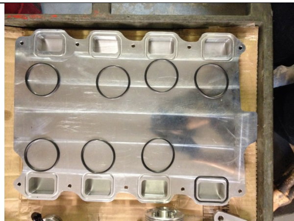
Figure 29: O-rings on bottom of intake tub.
