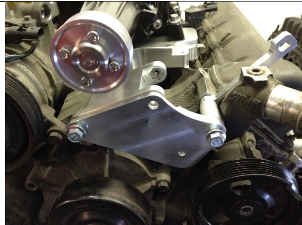
Figure 44: Alternator bracket installed.
