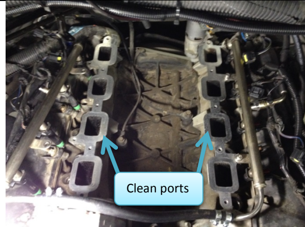
Figure 28: Clean intake ports.
