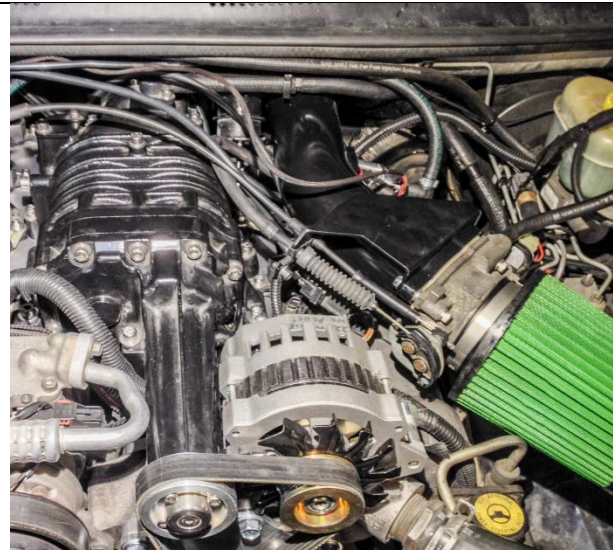
Figure 54: Throttle cables attached to bracket on intake tube.
