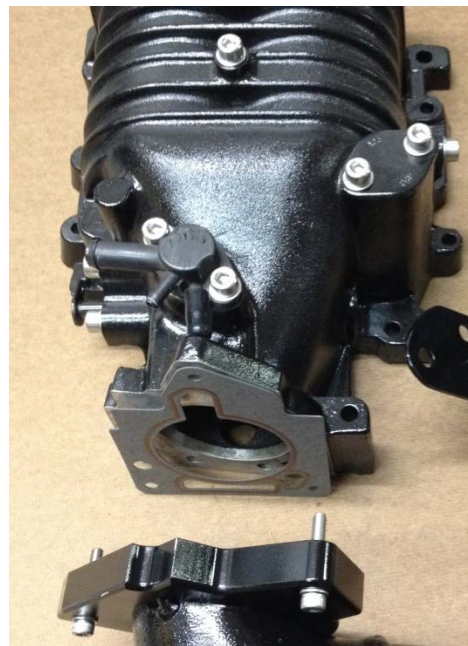
Figure 38: Supercharger intake gasket installed.
