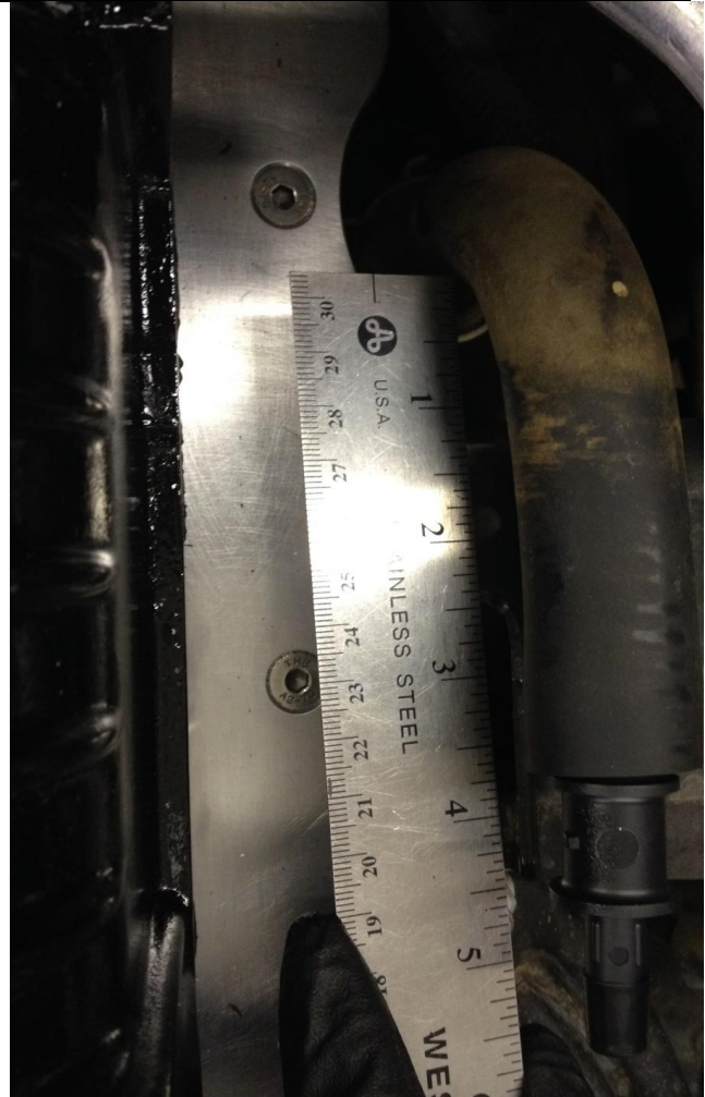
Figure 8: PCV hose cut and reducing connector installed.
