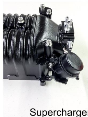
Supercharger with bypass valve attached
