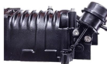
Supercharger with bypass valve attached
