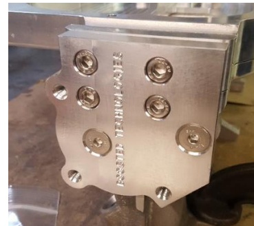
Figure 47: Torque power steering pump mount plate bolts last.
