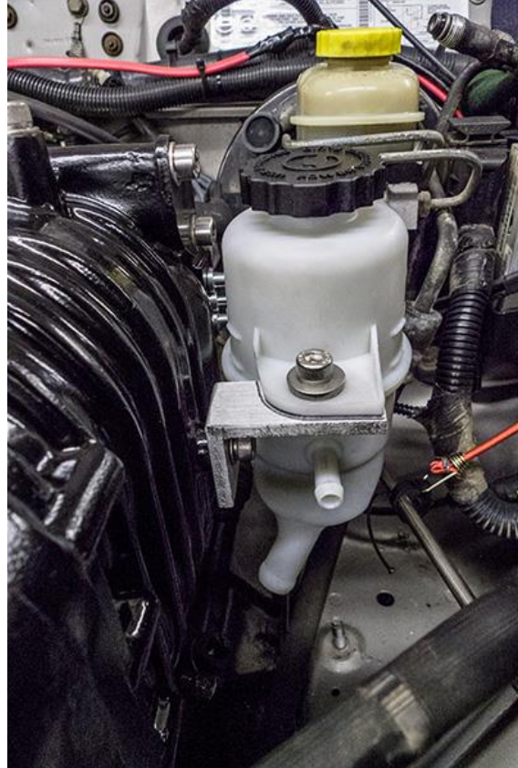
Figure 50: Power steering reservoir and bracket type 1.
