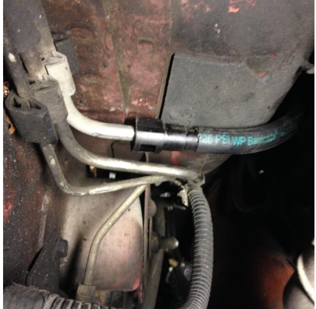
Figure 64: New fuel line connected to fuel line under driver side behind front tire.
