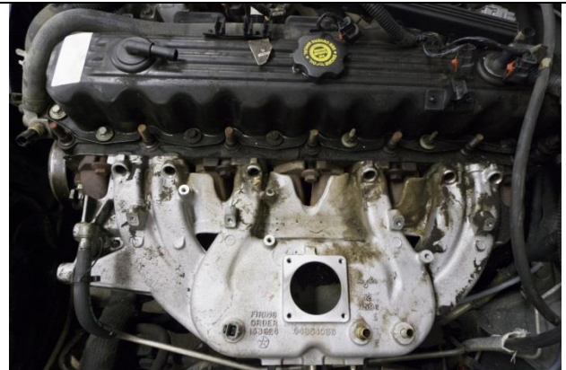
Figure 24: Intake manifold after removing heat shield.
