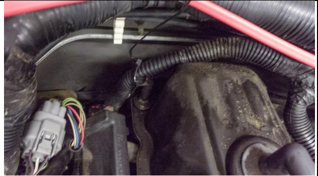
Figure 84: Wire tie down may hold loom too far toward passenger side for throttle body wire connection.
