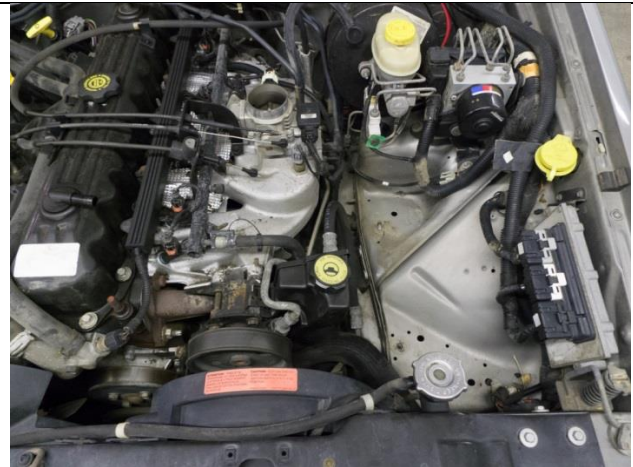
Figure 4: Stock air box and fresh air vent hose removed.
