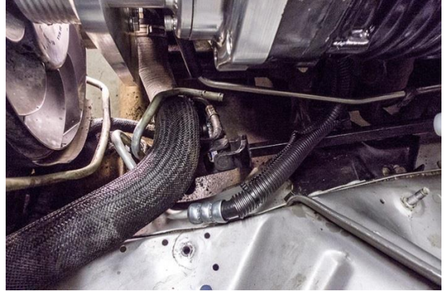
Figure 56: Stock power steering return line with tube removed and new high pressure line installed.
