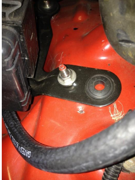
Figure 32: New hole to relocate front tab on ABS bracket.
