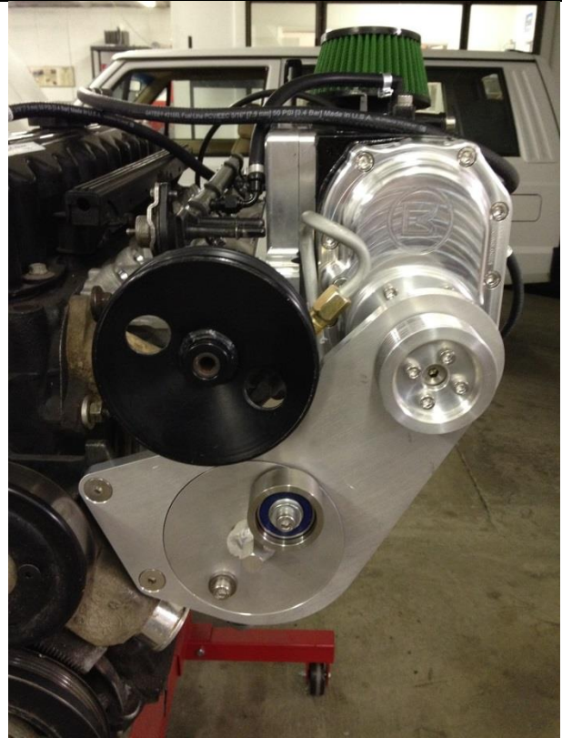
Figure 54: Nose support installed with tensioner disc.
