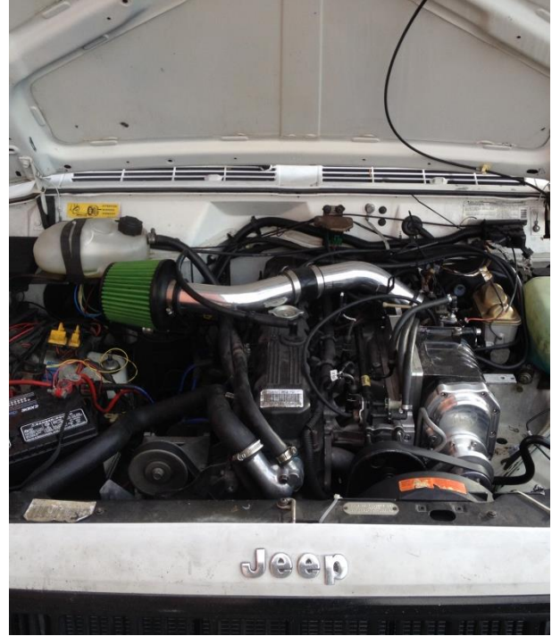
Figure 88: Air filter with aluminum elbows.
