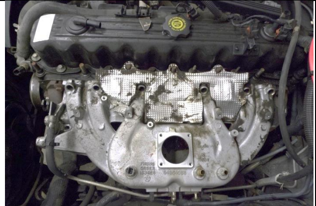
Figure 22: Intake manifold after fuel rail removal, wire housing moved and heat shield in place.
