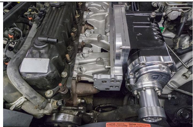
Figure 47: Torque power steering pump mount plate bolts last.
