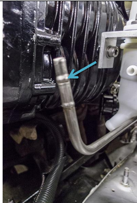
Figure 69: Stock fuel line with plastic/rubber end removed.
