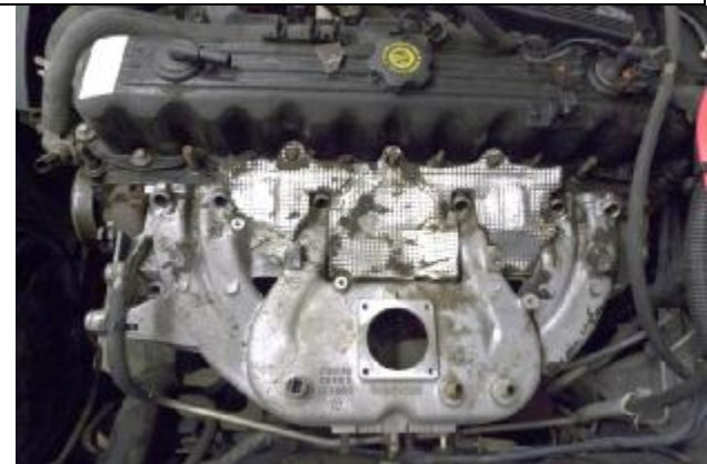
Figure 18: Intake manifold after fuel rail removal, wire housing moved and heat shield in place.
