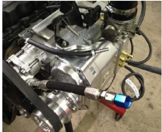
Figure 27: Power steering hoses installed and routed properly.
