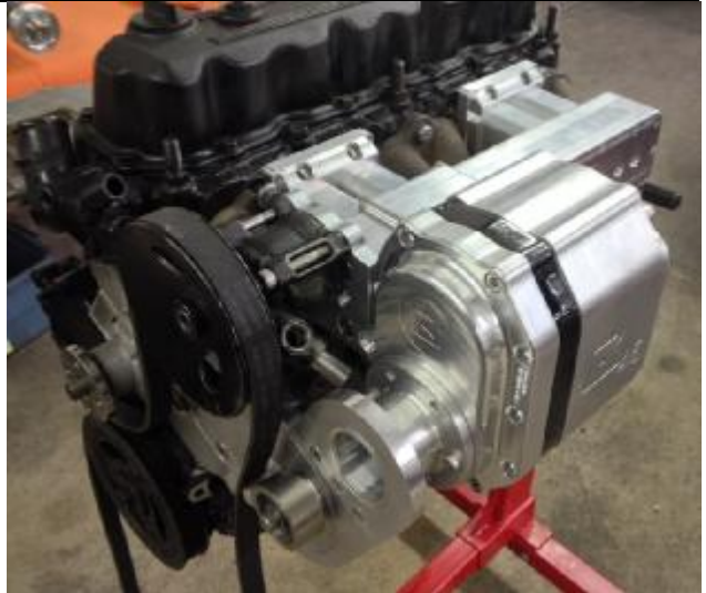
Figure 26: Power steering pump and supercharger nose support installed.
