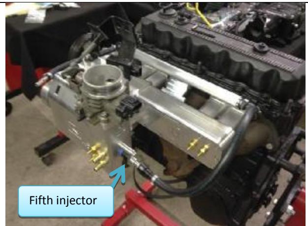
Figure 28: Fifth fuel injector installed on rear intake tube.
