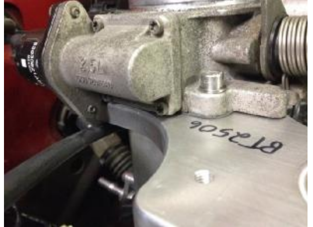
Figure 33: Throttle body sitting flush after removing protrusion.
