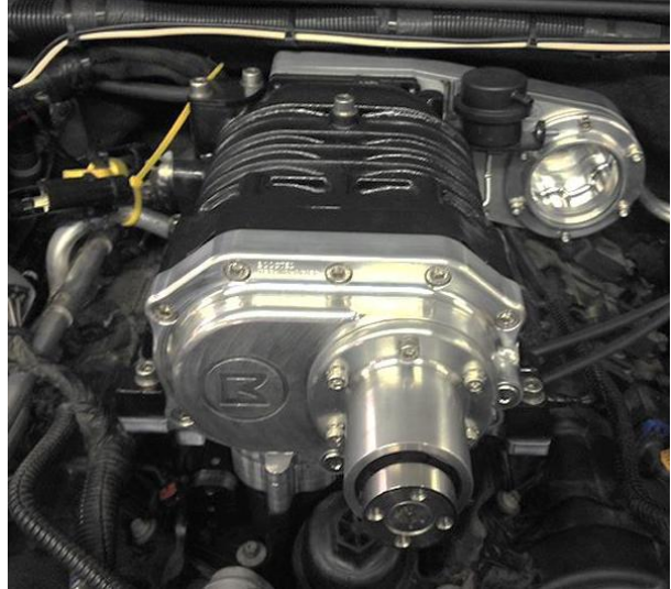
Figure 58: Supercharger installed on intake plate.
