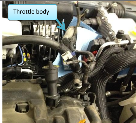
Figure 4: Throttle body placed behind ECU (on blue paper towel).
