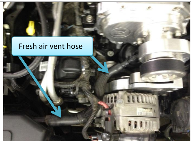
Figure 73: Fresh air vent hose routed under supercharger
