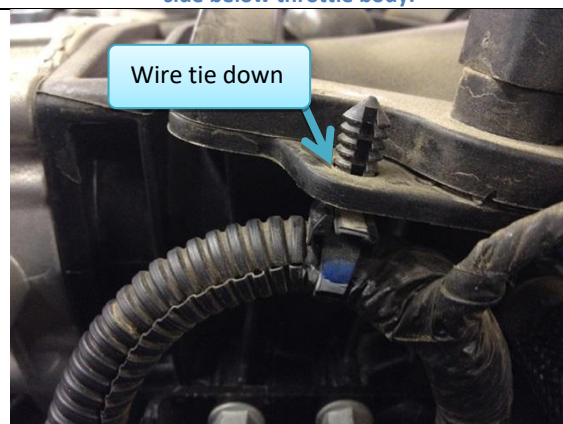
Figure 3: Wire tie down
