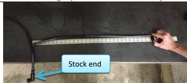
Figure 69: Valve cover vent and fuel vapor hose teed with stock end attached on short section.
