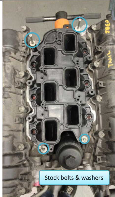
Figure 39: New intake manifold with four stock bolts.
