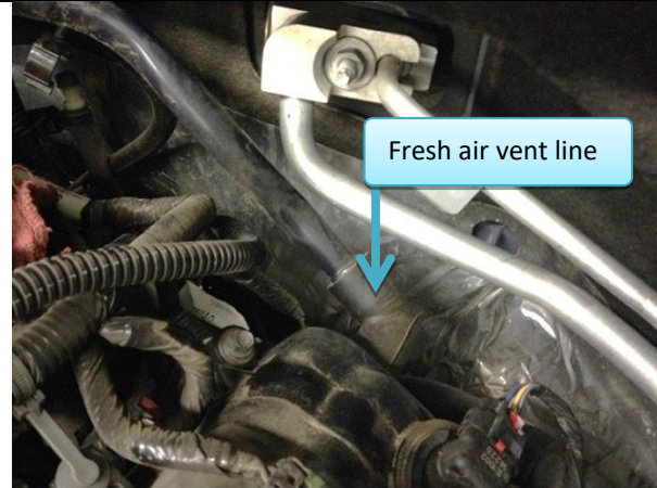
Figure 19: Driver side valve cover fresh air vent line connector.
