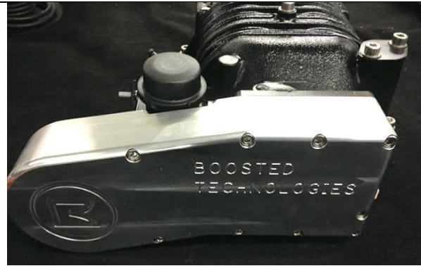
Figure 51: Rear intake housing installed on intake plate.
