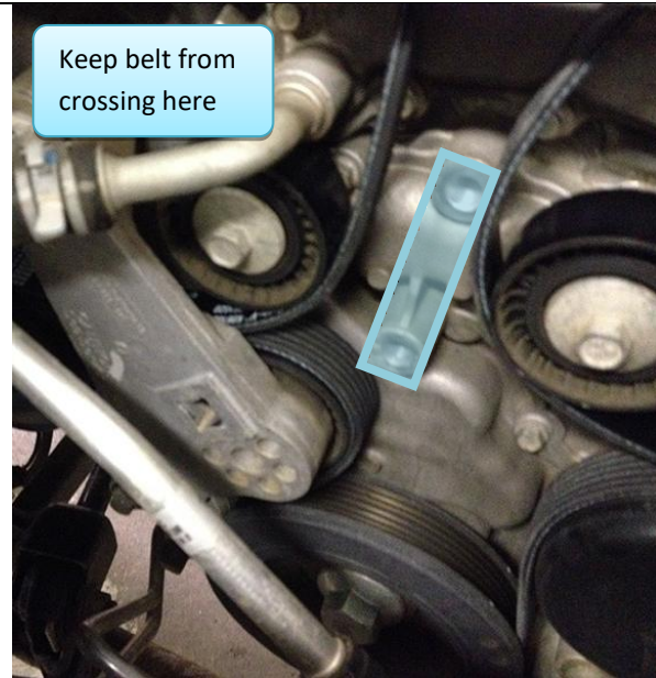
Figure 62: Serpentine belt properly routed with vertical section on either side of alternator support anchors.
